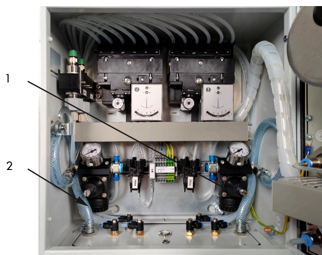
Fig. 19: Setup inside the Type 7311 Air Control System 1 Supply pressure regulator for control loop 2 (50R6) 2 Supply pressure regulator for control loop 1 (50R5)
