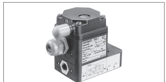
Fig. 1: 5/2-way solenoid valve · Actuated on one side · With spring return mechanism · K_{VS} 0.16 · G \frac{1}{4} connection
